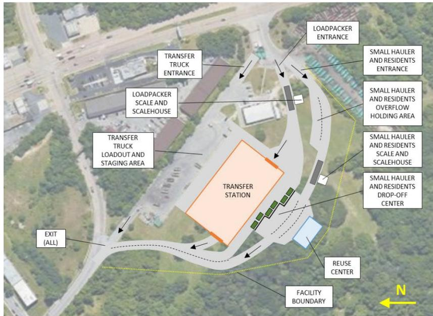
**Conceptual Layout of New Truck Transfer Facility at Bowleys Lane**
